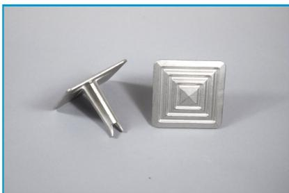
The stainless steel crossing studs are also 100mm square and have a serrated finish to improve skid resistance in adverse weather conditions, and have a fishtail shank.
